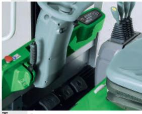
he ergonomic cab features the highest standards in operator comfort, safety and ease of access. The proportional electronic controls integrated in the new (optional) armrest enable the operator to manage all the hydraulic functions by simply moving the Mini-Joystick or Fingertips levers.
