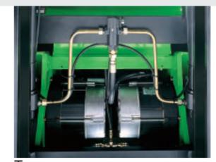
he new CESAB cenTAURO utilises two indipendent high power front wheel traction AC motors to form an electronic differential which allows it to work in the tightest spaces.
