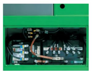
he electronic control unit, which is installed in the protected internal compartment, enables immediate access for programming and diagnostics. The truck performance characteristics can be adjusted to suit the working application and individual drivers needs.
