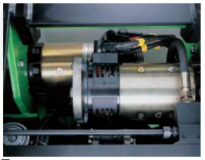
The powerful drive motors on both front wheels guarantee good performance and outstanding grip in all load and flooring conditions.
