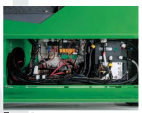
The MOSFET electronic control, housed at the side for easy access, allows modification of the drive and lifting parameters, as well as permitting counter-turning of the front wheels for lower turning radiuses.
