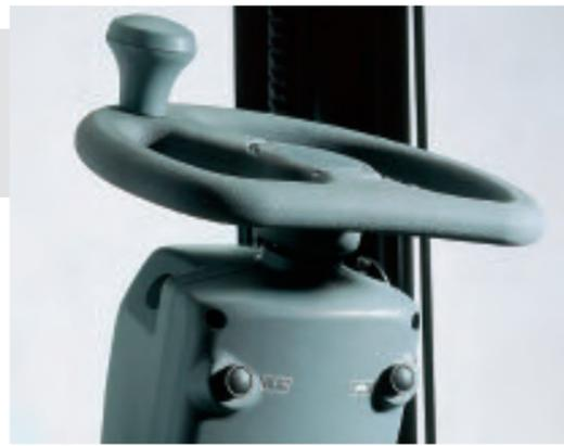
The operator has a choice of different driving-modes, selected by pressing the buttons on the steering column. Three options are available, from the high performance to the economy mode.
