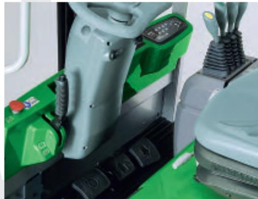
The ergonomic cab features the highest standards in operator comfort, safety and ease of access. The proportional electronic controls integrated in the new (optional) armrest enable the operator to manage all the hydraulic functions by simply moving the Mini-Joystick or Fingertips levers.
