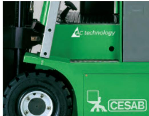
Excellent access to the driving seat, assisted by the large, conveniently located step with non-slip knurled aluminium tread.
